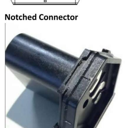
The solution was first verified empirically by machining connectors to varying notch dimensions and measured pre- and post-crimp. Significant reduction in connector growth was found:
